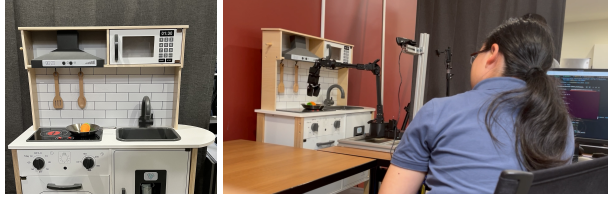
Figure 7: (Left) Closeup view of the kitchen set with the spoon hanging on the wall, above the pan on the stove. (Right) WidowX 250 6DOF robot arm, user, and text prompt for experiments.
