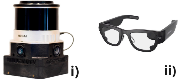
Fig. 2: These two Oxford-based datasets use these multi-sensor perception units for data recording i) Frontier and ii) Meta Aria glasses.
