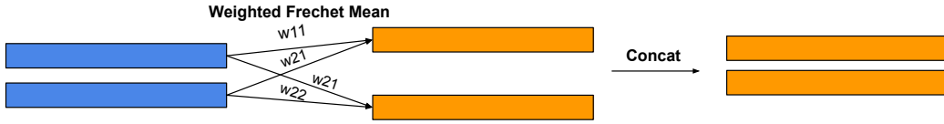
Figure 8: Weighted Riemannian Pooling: Performs multiple weighted Fréchet means on the channels of the input SPD
