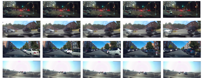
Fig. 6. (Row-1,2) True Positives, i.e. failures detected correctly by our method. (Row-3,4) False Negatives, i.e., actual failures detected as safe by our method.
