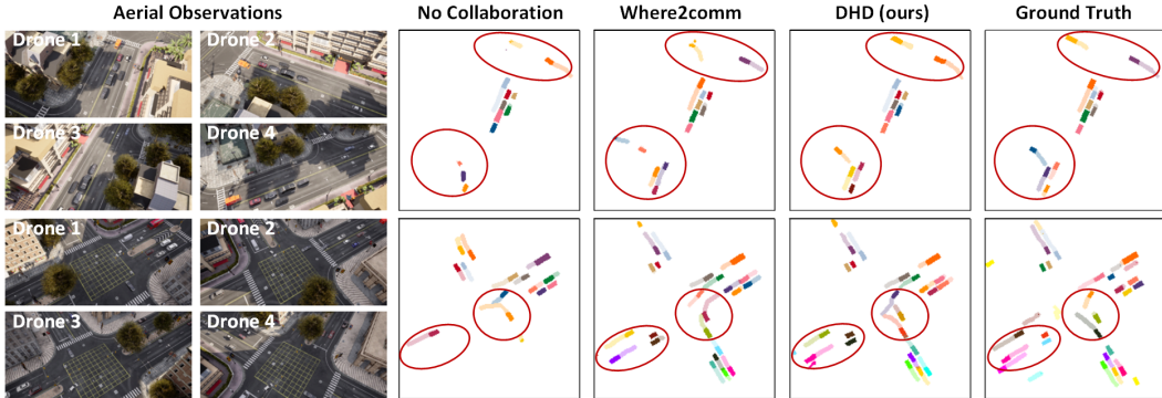
Figure 7: A comparative analysis of visualizations among various collaboration baselines. Each instance is allocated a distinct color, and its predicted trajectory is represented with the same color and slight transparency. Red circles highlight the areas where other baselines make mistaken predictions.
