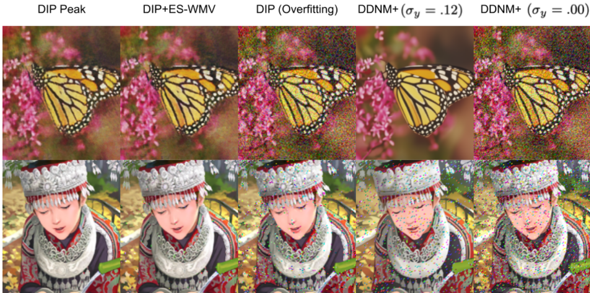
Figure 11: Visual comparisons for 2\times image super-resolution task with additional noise. Top row: with additional low-level Gaussian noise; Bottom row: with additional low-level impulse noise.
