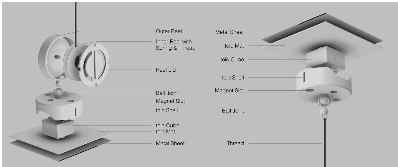
Figure 2: (Left) The setup of a floor toio robot and (Right) the hardware setup of a ceiling toio.
