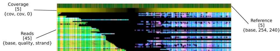
Figure 1: 201 \times 55 pixel pileup image. Feature rows are labeled by brackets and RGB channels are labeled by curly braces. Reference rows are encoded in R channel by base A: 250, G: 180, T: 100, C: 30, N: 0. Coverage rows are encoded in RG channels by the number of mapped reads covering each position. Reads are encoded in RGB channels by base types, base quality, and strand directionality positive: 70, negative: 240.
