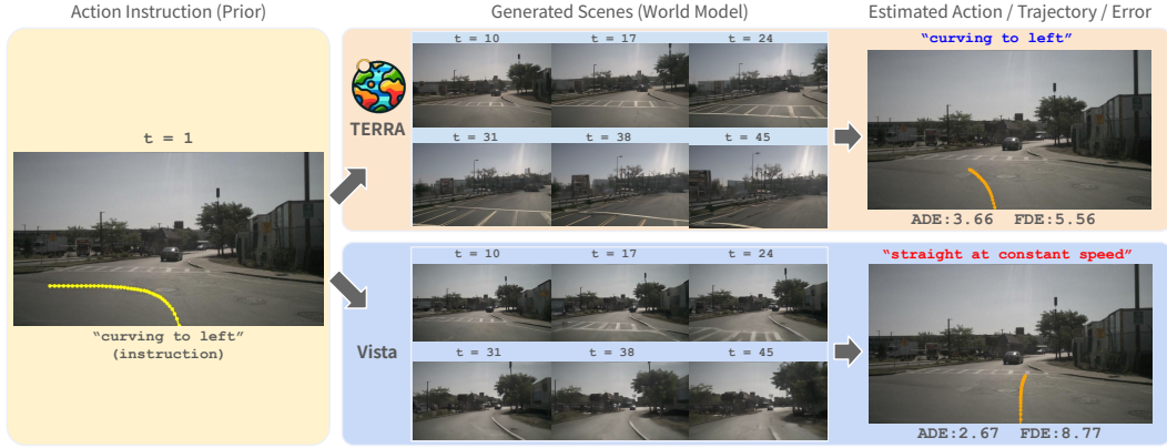
Figure 1: ACT-BENCH assesses the action controllability of world models by estimating actions, trajectories, and their deviations from the generated driving scenes using our motion estimator, ACT-ESTIMATOR. In the upper example, TERRA successfully follows the instruction to “curving to left.” In contrast, the lower example illustrates that Vista fails to follow the instruction.
