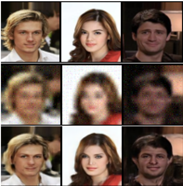
Figure 6: CelebA64 SR 4X from 16 \times 16 to 64 \times 64 order: Ground truth, Input image, Output image
