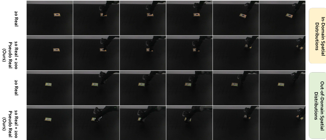
Figure 5: Visualization of DP performance on Move Playing-Card Away . Top two rows: objects lie initially within the region predefined in collected real-world demonstrations (in-domain spatial distribution). Bottom two rows: initial positions are outside the region (out-of-domain spatial distribution). Policies shown are trained under 20 Real and 10 Real + 200 Pseudo Real , respectively.
