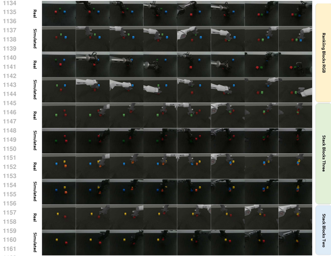
Figure 11: Real2Sim alignment on additional tasks. From top to bottom: Ranking Blocks RGB , Stack Blocks Three and Stack Blocks Two .
