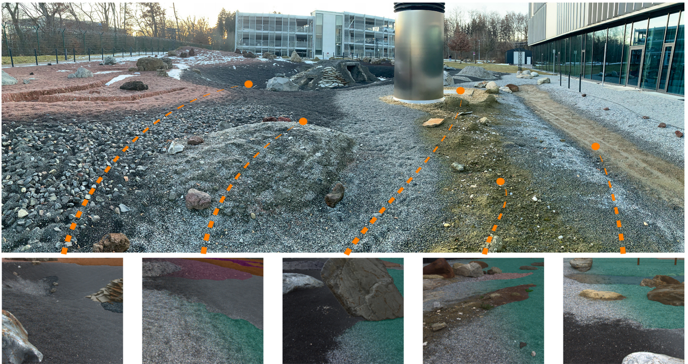
Fig. 5. Image of the planetary exploration outdoor laboratory and example samples from the EXTerra dataset with partially overlaid annotations and the approximate capture locations indicated by orange lines.
