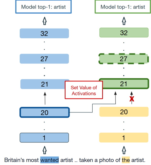
Figure 4. By injecting the output from the top-1 saturation layer of “the” as input to the subsequent layer of “artist”, we trigger a saturation at the injected layer (21) in the post-intervention run, without altering the top-1 prediction. Saturation layers are marked in bold, saturation layer in the original run for “the” token marked with dashes. The use of activations from adjacent layers is not depicted for the sake of clarity.
