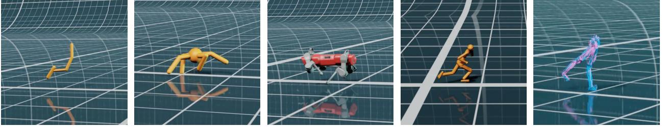
**Figure 7. Experimental Environments.** Locomotion tasks in increasing order of action space ( $m$ ) dimensions (left to right): Hopper ( $m = 3$ ), Ant ( $m = 8$ ), Anymal ( $m = 12$ ), Humanoid ( $m = 21$ ) and SNU Humanoid ( $m = 152$ ).
