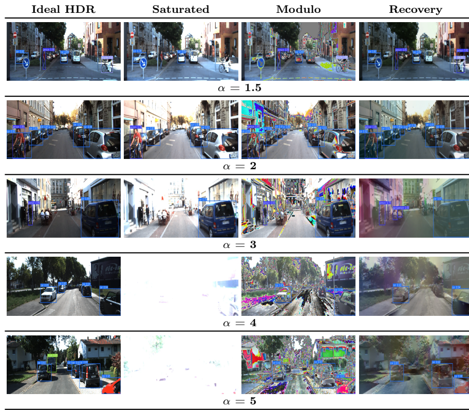
Fig. 2: Comparison of imaging techniques under varying levels of light saturation. Each column stands for; Ideal HDR, Saturated, Modulo, and Recovery. Each row shows the results for different values of the saturation factor \alpha , ranging from 1.5 to 4.
