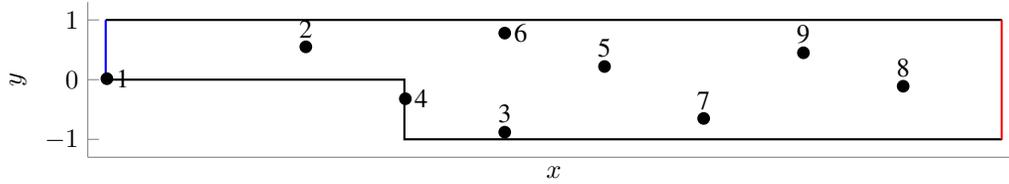
**Figure 15:** Spatial location of the 9 random chosen evaluation points. Point 1:  $(-4.98, 0.016)$ , Point 2:  $(-1.65, 0.55)$ , Point 3:  $(1.68, -0.88)$ , Point 4:  $(0.016, -0.32)$ , Point 5:  $(3.35, 0.22)$ , Point 6:  $(1.68, 0.78)$ , Point 7:  $(5.01, -0.65)$ , Point 8:  $(8.35, -0.11)$ , Point 9:  $(6.68, 0.45)$
