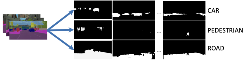
Figure 2: Construction of multiple binary segmentation datasets from one semantic segmentation dataset. Each image-mask pair in the semantic segmentation dataset is divided into multiple image-mask pairs for binary segmentation, one for each class present in the semantic segmentation.
