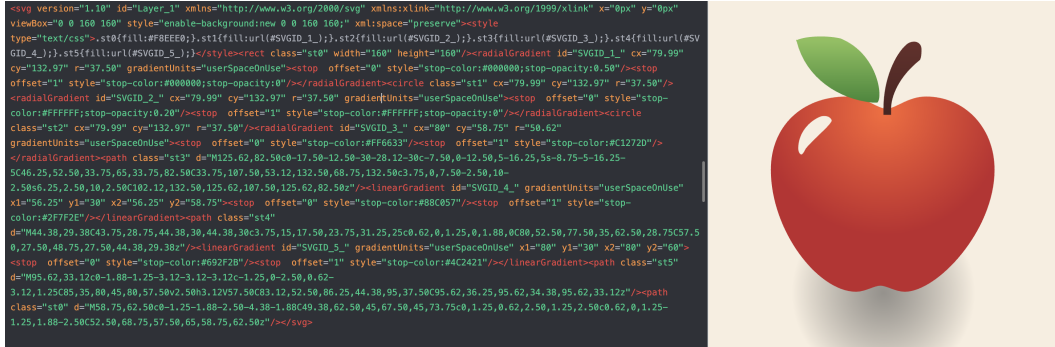
Figure 12: Im2SVG Vectorization Result: Apple Example This challenging sample highlights the effectiveness of RLRF. The image contains complex shapes, lighting effects, and semantic cues that require multiple SVG primitives: rectangles for the background, paths for the main structure, and gradients for shadows and highlights. Such examples are not present in the SVG-Stack dataset, which primarily contains simpler icons and logos. While SFT alone fails to reproduce this image, RLRF enables the model to generalize and successfully generate high-fidelity SVGs for out-of-distribution samples like this.
