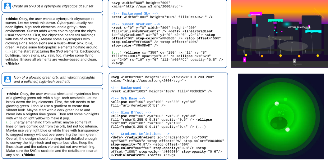
Figure 9: Text2SVG Generation Examples from RLRF. We show samples generated by the Qwen3-8B model after applying RLRF training. Each example begins with a reasoning-style planning phase, followed by the generation of SVG code. The two prompts—one describing a cyberpunk scene at sunset and another depicting a mysterious green orb—are rendered into long and complex SVGs that closely match the inputs. Notably, the model achieves this despite its relatively small size (8B), and such quality was not attainable before reinforcement learning. Larger models and more training data are expected to further improve results, as current trends show no signs of saturation.
