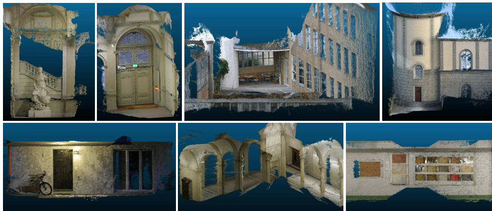
Figure 14: Point Clouds of scene dataset ETH3D (Schops et al., 2017) reconstructed by MVSFormer.
