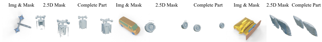
Figure 5: 3D part amodal segmentation on generated objects and scanned objects from OmniObject3D . Our method seamlessly integrates with arbitrary zero-shot 3D part segmentation models. We can generate even precise joint structures , such as the mortise-and-tenon joints at the robot’s connections shown in the figure.
