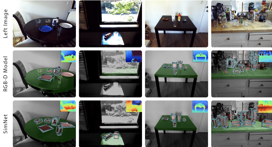
Figure 4: Graspable Object Predictions: SimNet is evaluated on an OBB regression task with objects of varying sizes and shapes on flat surfaces. Top: The left RGB image from different homes. Middle: Our model prediction trained with RGB-D sim-to-real transfer similar to [4]. The top right corner is the output of the Asus Xtion depth sensor. Bottom: SimNet. In the top right, we show the low-res disparity estimate predicted by the learned stereo net. SimNet consistently enables better sim2real transfer of the predictions for optically challenging scenarios.
