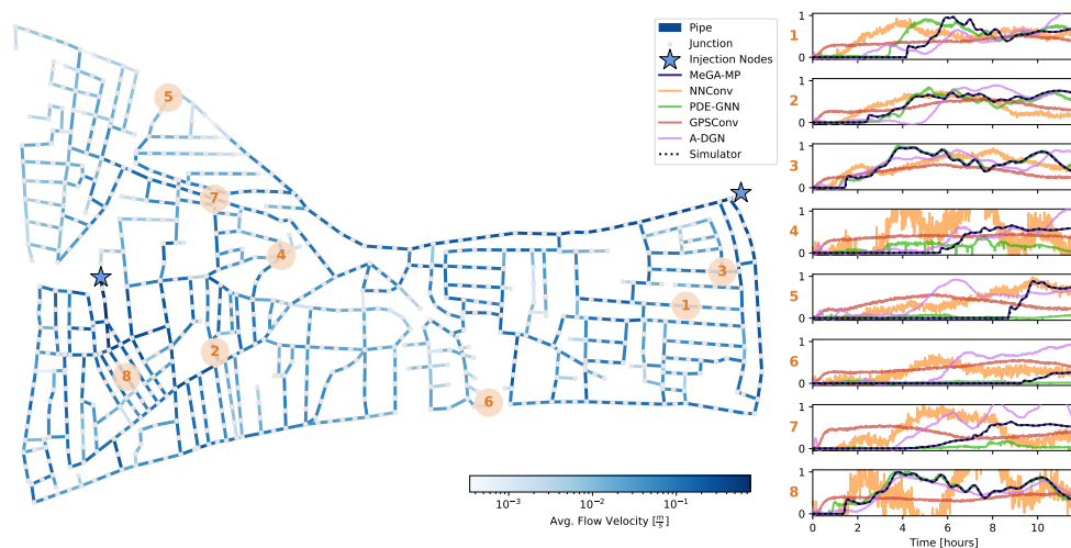
Figure 6: Predictions of baselines and MeGA-MP for the advection dynamical system at a randomly chosen subset of nodes of the WDS L-Town . The L-Town metric graph is not part of the training set. Edge color corresponds to the flow velocity averaged across all time steps of the sample.
