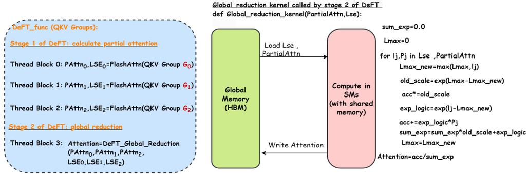
(a) Left: Illustration of DEFT Attention Kernel with two stages. Right: Global reduction kernel called in DEFT stage 2 illustrated in Figure 10b. QKV Groups  $G_0, G_1$  and  $G_2$  are from DEFT QKV groups in Figure 3.
