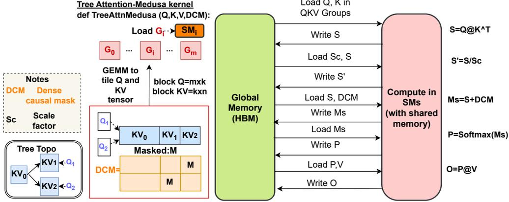
Figure 8: Operations of Tree Attention-Medusa (Cai et al., 2024). No *Kernel Fusion* or *Tiling* strategy is applied, which introduces significant IO of partial results like  $QK^T$ , DCM, and Softmax between GPU global memory and on-chip shared memory.
