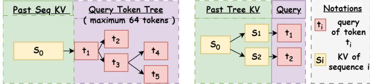
(a) (Left) Sequence KV with queries in a tree for parallel decoding (Miao et al., 2023; Cai et al., 2024), where a *causal mask* is applied to record the causal information among queries in a tree of tokens. (Right) Tree KV with parallel queries for shared prefixes in multi-step reasoning.
