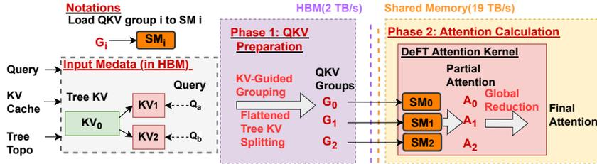
Figure 2: **Overview of DEFT.** *Input Metadata* is prepared in the system elaborated in Appendix A.1. In *QKV Preparation Phase* (see Section 3.3), the QKV will be grouped logically to partitions with IO-awareness of shared prefixes’ KV cache and load-balancing. These partitions will guide the loading of QKV on the *Attention Calculation Phase* (see Appendix A.4), where the attention calculation will be executed.
