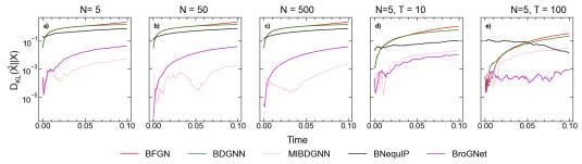
Figure 5: Trajectory roll-out error of BFGN, BDGNN, MIBDGNN, BNequIP and BROGNET trained on N = 5 and T = 1 to unseen system sizes (N = 50, and 500) and unseen temperatures (T = 10 and 100) on the linear spring system. The plots are obtained based on 100 forward simulations by the trained model with random initial conditions.
