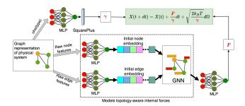
Figure 1: BROGNET's architecture. MLP refers to multilayer perception, GNN to graph neural networks and ohe to one-hot encoding.
