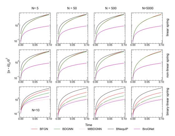
Figure J: Position error of BFGN, BDGNN, MIBDGNN, BNequIP, and BROGNET trained on N = 5 system and tested on N = 50, 500, 5000 for linear (row 1), non-linear spring (row 2), and binary linear spring (row 3) systems evaluated on 1000 forward trajectories.
