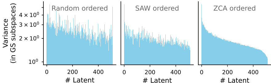
Figure 3: Latent unit variances in our subspace after Gram-Schmidt orthogonalization of layer 12 from VGG-16. Prior to the orthogonalization, the units are ordered either randomly (left), ordered using the SAW importance measure (middle) and ordered using our proposed ordering by unnormalized-ZCA variances (right).
