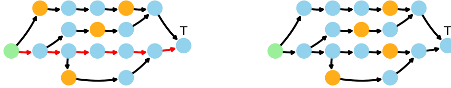
Figure 1: Positive (left) and negative (right) GLoRa examples for d = 6 : green (i.e., source), blue (normal), and orange (hole) nodes have embeddings of form [1, -] , [-, 1] , and [-, 0] , respectively; T marks the target node; the red-arrows chain is the long-range dependency path
