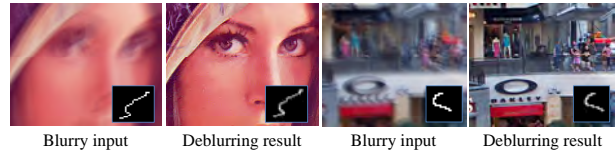
Figure 9: Deblurring of synthetic examples. The first and third images show blurred images with applied motion blur kernels. The second and fourth images show our deblurring results with estimated kernels. The kernel sizes of the left and right examples are 29 \times 25 and 21 \times 21 , respectively.
