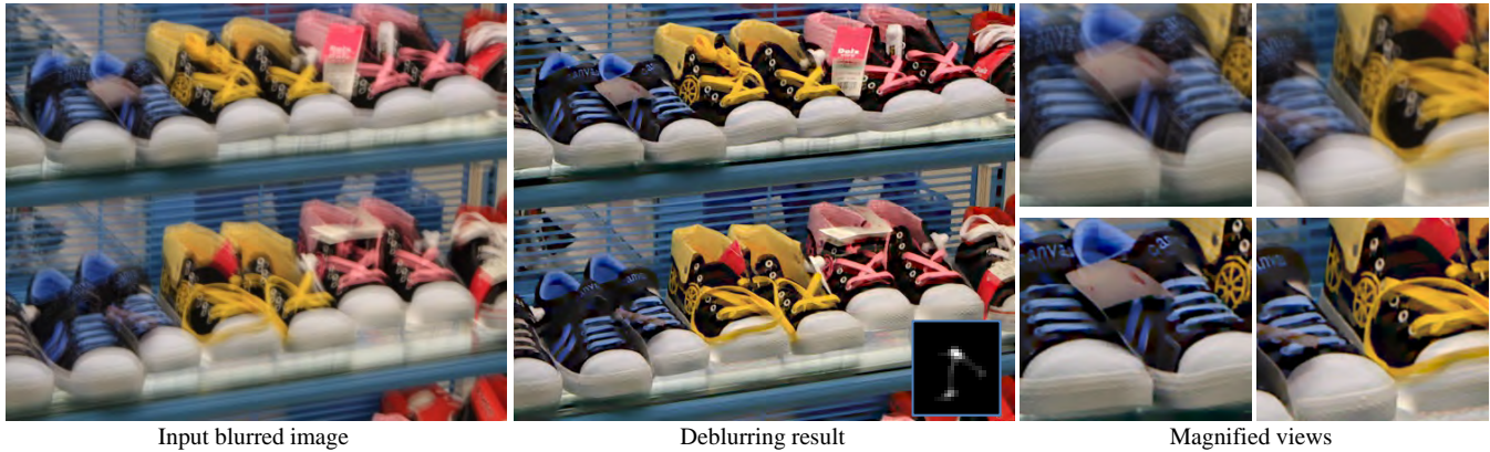
Figure 1: Fast single image deblurring. Our method produces a deblurring result from a single image very quickly. Image size: 713 \times 549 . Motion blur kernel size: 27 \times 27 . Processing time: 1.078 seconds.
