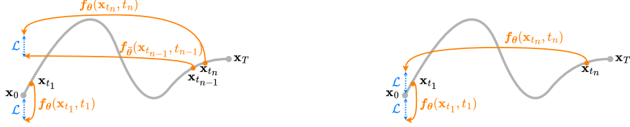
Figure 1: CMs (left) are weakly supervised ODE solvers, only learning to map points along a trajectory that are near the trajectory’s origin back to the origin itself; points that are far from the origin instead enforce a self-consistency property, relying on weak self-supervision to solve the PF ODE. Direct CMs (right) are strongly supervised ODE solvers, instead learning to directly map all points along a trajectory back to the origin.
