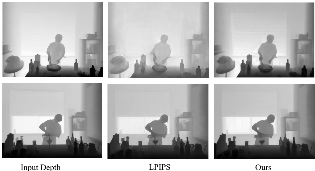
Figure 13: A visual comparison of rendered depth maps using the perceptual depth loss and our ordinal depth loss.
