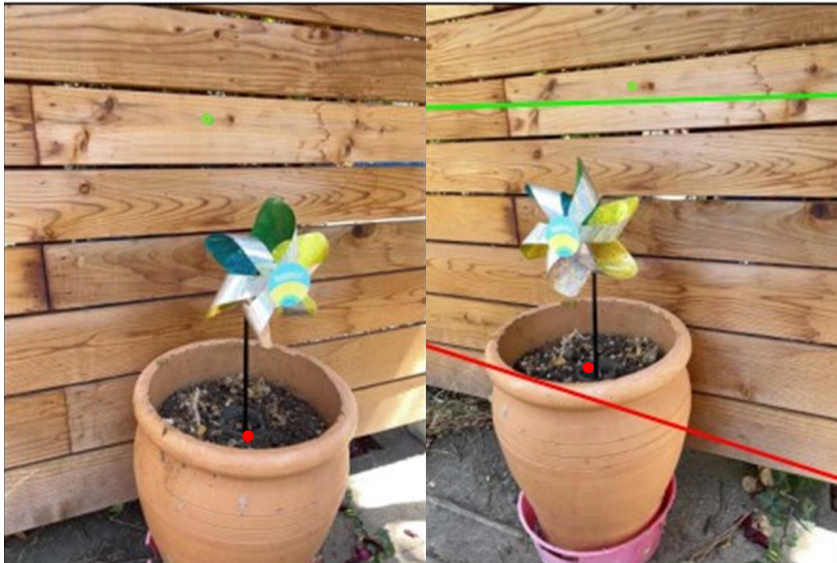
Figure 9: We provide a pair of images on the iPhone (Gao et al., 2022) dataset. We draw two correspondences in the same color and their corresponding epipolar lines that are computed from the provided camera poses. The epipolar lines deviate far from the correspondences, which demonstrate that the camera poses are not accurate enough.
