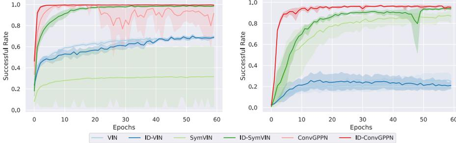
Figure 7: **(Left)** Training curves on 2D maze navigation  $15 \times 15$  maps, with 80 layers for explicit planners and 80 iterations for implicit planners. **(Right)** Training curves on  $49 \times 49$  maps, with 30 layers for explicit planners (due to scalability issue) and 80 iterations for implicit planners.
