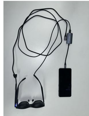
Figure 2: Hardware used for data collection and model testing. The event-camera is mounted on the left side of the glasses, with the display connection on the right.
