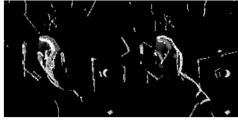
(b) Example time surface with left hand side illustrating the positive polarity image and right hand side illustrating the negative polarity image.
