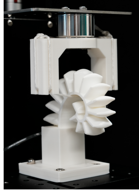
Fig. 3. Hardware setup for the holding force test.
