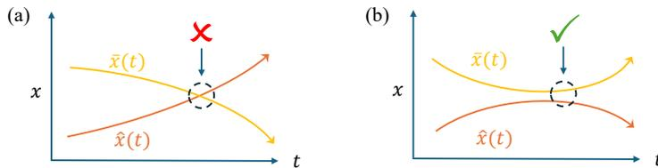
Figure 6. Illustration of the non-intersecting trajectories of ODEs. (a) The two trajectories intersect each other, which is not feasible for ODEs. (b) Any two trajectories cannot intersect each other at any time  $t$ .
