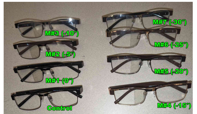
Figure 2: Model glasses. Labels are model numbers with ideal perceived location of display combiner edge. We use negative values to indicate offsets from PPOG towards the nose.
