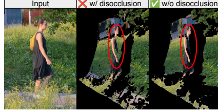
Figure 10: We mask out the disoccluded region (right) to prevent potential see-through artifacts (middle).
