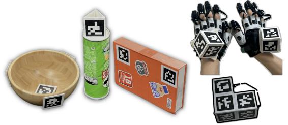
Fig. 4: Objects used in the experiment and a marker system for 3D tracking.
