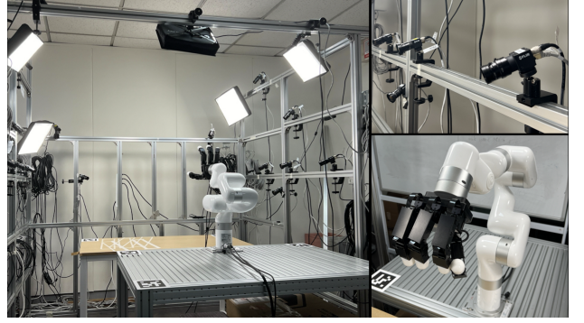
Fig. 3: System Overview: Our system consists of 16 synchronized cameras, an xArm6 robot arm, and a 16-DoF Allegro robot hand.
