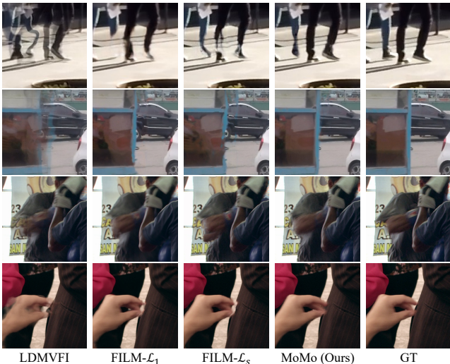
Figure 5: Qualitative comparison against state-of-the-art methods on ‘extreme’ subset of SNU-FILM and Xiph-4K. Our results show the least artifacts and generate well-structured images.
