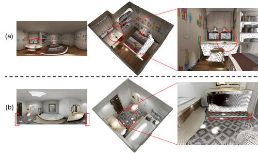
Figure 7: DA 2 ’s limitations. (a) The white lamp’s predicted distance is mistakenly aligned with the desk surface. (b) Visible seams appear along the predictions at lower left–right boundaries.
