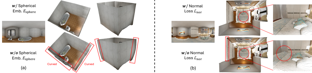
Figure 6: Ablation studies of DA 2 . (a) Removing the spherical embedding E_{\text{sphere}} causes curved, distorted geometry. (b) Omitting the normal loss \mathcal{L}_{\text{nor}} yields rougher surfaces and more artifacts.
