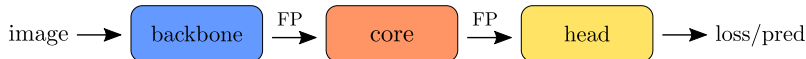
Figure 1: High-level view of a computer vision network. The backbone ( left ) processes the image to output a set of feature maps ( i.e. a feature pyramid). The core ( middle ) takes in a feature pyramid (denoted by FP) and returns an updated feature pyramid. Finally, the head ( right ) produces the loss during training and makes predictions during inference from the final feature pyramid. In this work, we focus on improving the core.
