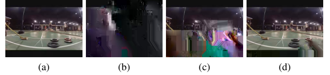
Fig. 6: Example of 4 different levels of distortion for an H.265 packet, comprising an intra frame, where a single bit is inverted. Each example corresponds to an inverted bit occurring at a different position, in percentage, within the packet (0% is the first bit and 100% the last): (a) original image, (b) inverted bit at about 30%, (c) inverted bit at about 40%, (d) inverted bit at about 70%.
