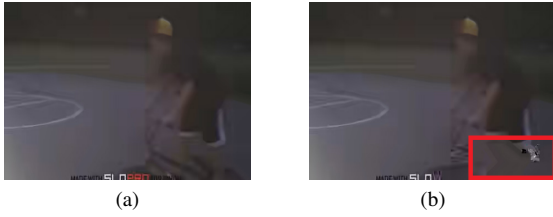
Fig. 8: (a) Intact intra image after H.265 decompression (QP=37). (b) A candidate image on which a bit is inverted at the end of the packet (random position at about 90%).
