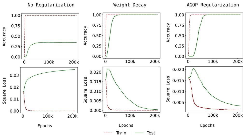
Figure 8. One hidden layer fully connected networks with quadratic activations trained on modular addition with  $p = 61$  with vanilla SGD. Without any regularization the test accuracy does not go to 100% whereas using weight decay or regularizing using the trace of the AGOP result in 100% test accuracy and grokking.
