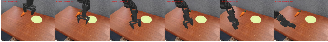
Figure 6: Failure case: The robot arm failed to reach the source object carrot using OpenVLA base.
