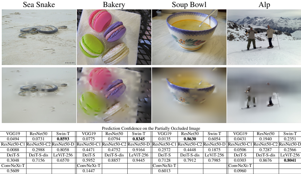
Figure 6: Qualitative Cross-Testing Results. The partially occluded images were generated using iGOS++ heatmaps on the algorithm with bolded number (not necessarily the highest). Then the same image is tested on multiple networks and we show predicted class-conditional probabilities on the ground truth class (written above). It can be seen that global attention models sometimes obtain high confidence when shown a small combination of regions, and CNN confidences vary greatly depending on whether certain features were observed. (Best viewed in color)
