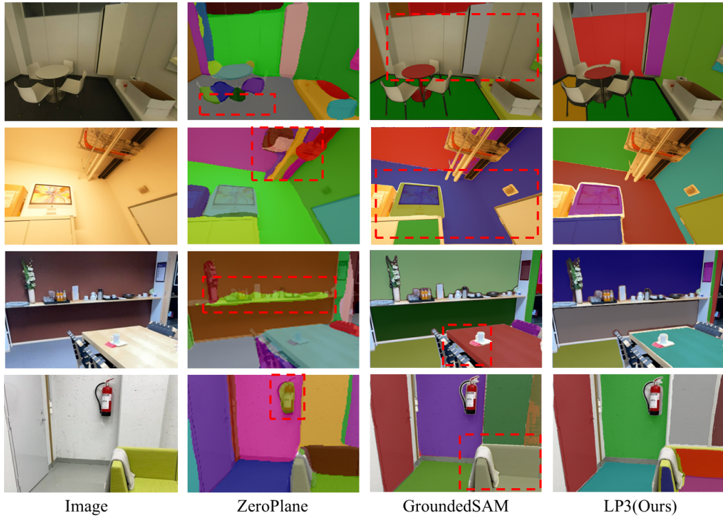
Figure 12: Comparison of planar priors. ZeroPlane fails to distinguish fine details or curved surfaces as non-planar regions, while GroundedSAM suffers from plane omission and merges planar regions.
