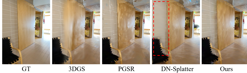
Figure 4: Novel view synthesis comparison. With the introduction of planar and geometric supervision, PlanarGS can effectively eliminate artifacts present in other methods.
