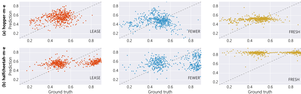
Figure 3: The comparison between prediction value by the learned rewards and their ground truths for different methods under (a) hopper-medium-expert and (b) halfcheetah-medium-expert datasets, where the value predicted by the trained reward model and ground-truth reward value are both normalized to [0, 1] . From left to right are methods LEASE, FEWER and FRESH, respectively.
