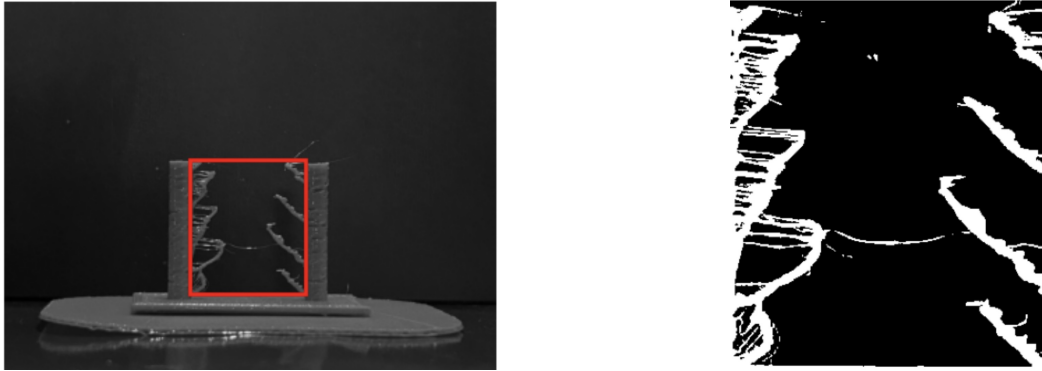
Figure 10: Grayscale image (BO, iteration 2) of the printed part with the region of interest (left panel), and white pixels approximating the stringing amount (15.9%) over the region of interest (right panel).
