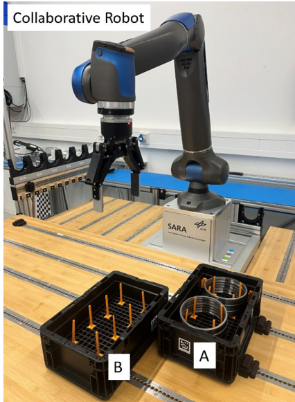
Figure 1: The experimental setup is composed of a torque-controlled, 7-DoF, robot mounted on a manufacturing workstation, boxes A and B, which contain inside them the rings that have to be picked from A and placed to B.
