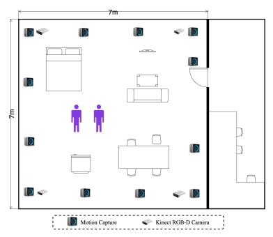
Figure 6: Layout of the data collection environment. The  $7m \times 7m$  capture area (left) is surrounded by sensors. The workstation (right) is located outside the sensors' field of view, allowing researchers to monitor the process and instruct subjects. The furniture positions shown are illustrative, as the scene layout was frequently changed.
