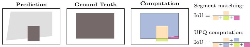
**Fig. 6:** UPQ computation between a prediction containing an instance (black), ANY region (gray), and background (white), and a ground-truth instance (black). For segment matching, the ANY regions are ignored, which leads to an  $\text{IoU} > 0.5$  in this example. Before UPQ computation after matching, the matched ANY regions are replaced with the ground truth.
