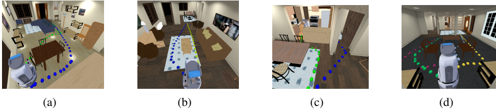
Figure 2: Examples of single-image trajectory trails in 4 scenes: a) move towards the door; b) move to the table in the kitchen; c) move to the table; d) move to the shelf behind the columns.
